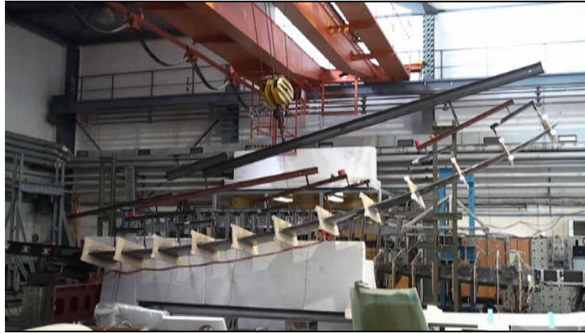
Figure 1.1: A strength test of glider wing at IAE Brno University of Technology
