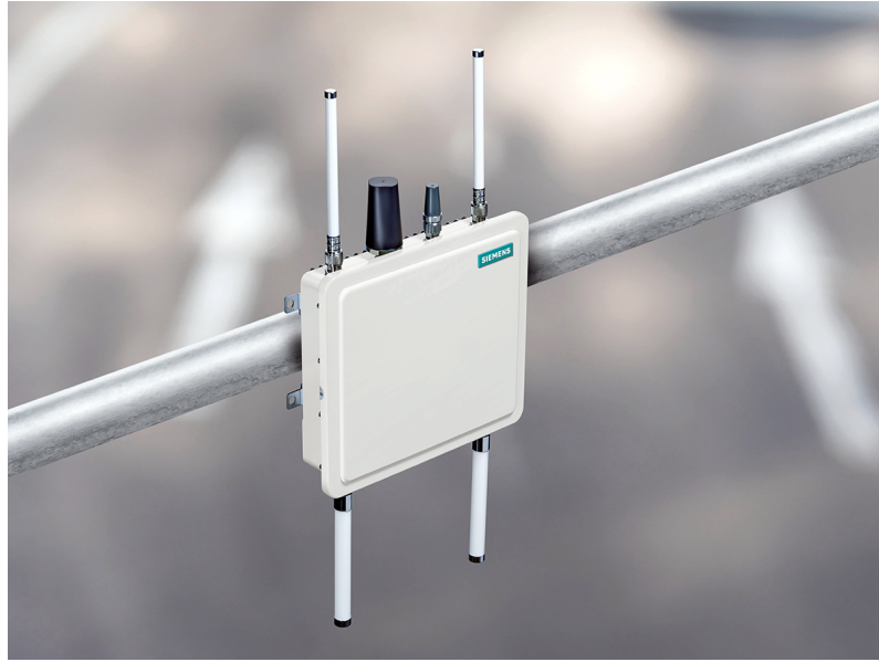
Fig. 1.4: Road Side Unit from company Siemens ITS [35].
