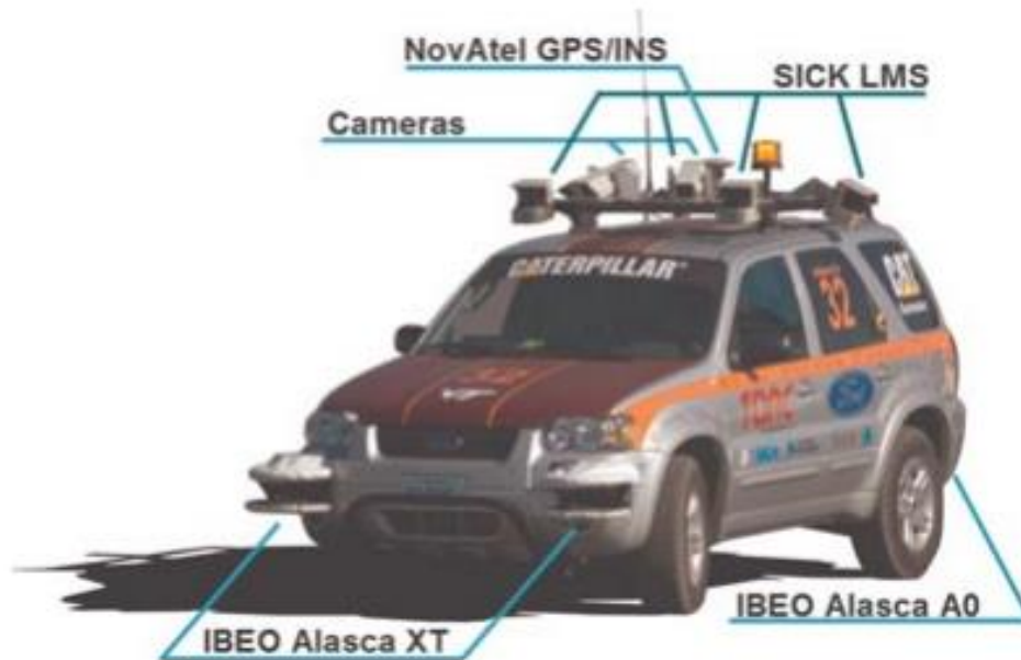
Figure 7 Odin- mounting locations of sensors (Source: Bacha A., et.al. (2008). Odin: Team VictorTango's Entry in the DARPA Urban Challenge. in Journal of Field Robotics 25(8), 467–492 (2008).)
