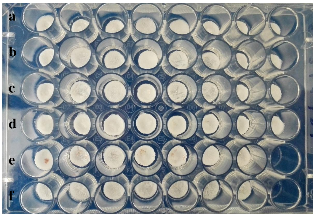
Appendix 2: The second serie of the samples, where each line contains the same type of samples – Coll (a), Coll/Chit (b), 1_Coll/Chit_SeCh (c), 1_Coll/Chit_SeB (d), 5_Coll/Chit_SeCh (e), 5_Coll/Chit_SeB (f).
