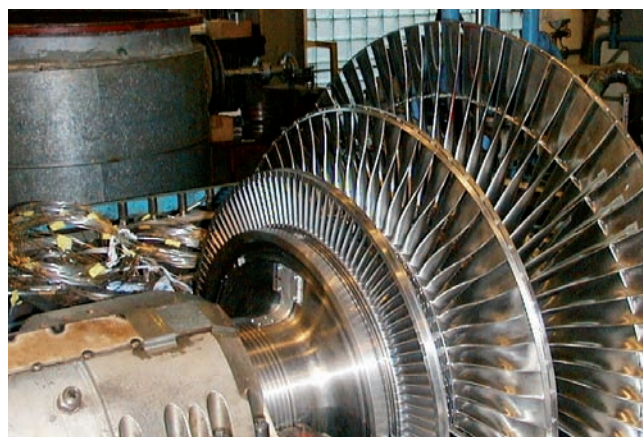
LP rotor in model test turbine Verification of calculation results, a central part of Alstom R&D
