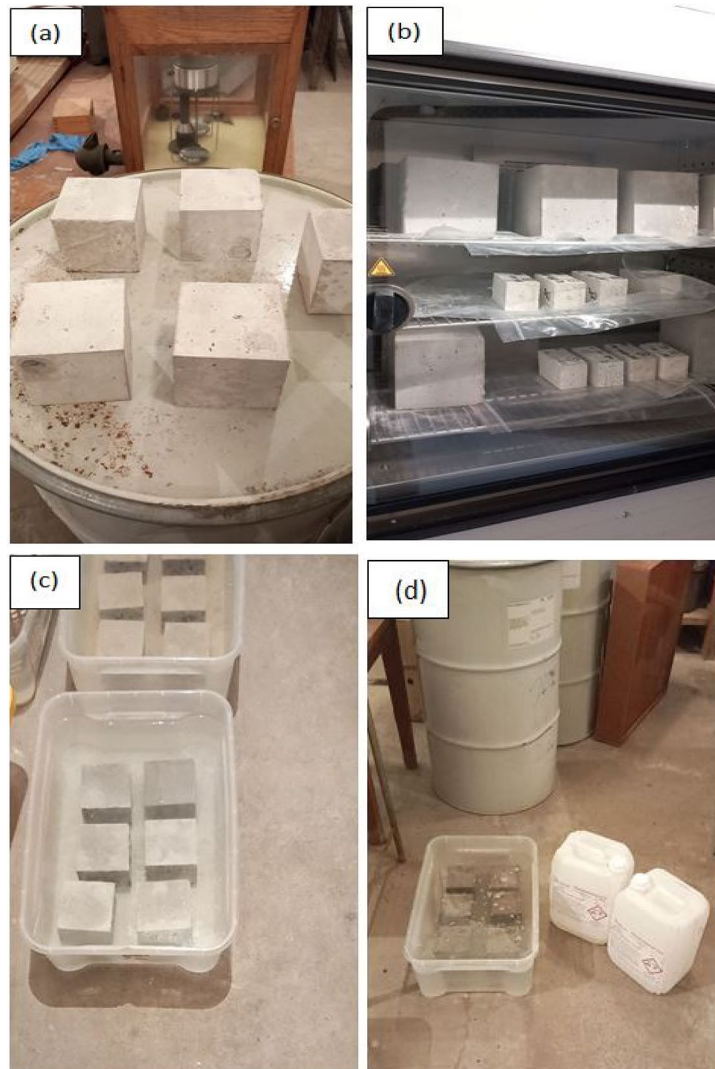
Fig. 5. Different curing methods after exposure to 600 °C: (a) Air-; (b) CO 2 -; (c) water-; and (d) water glass-curing.
