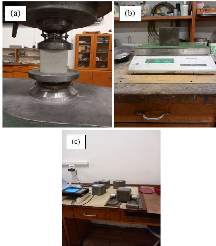
Fig. 3. (a) Compressive strength, (b) dry density, and (c) ultrasonic pulse velocity test setup.
