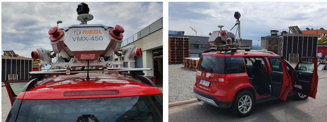
Figure 1. RIEGL VMX-450 configuration
