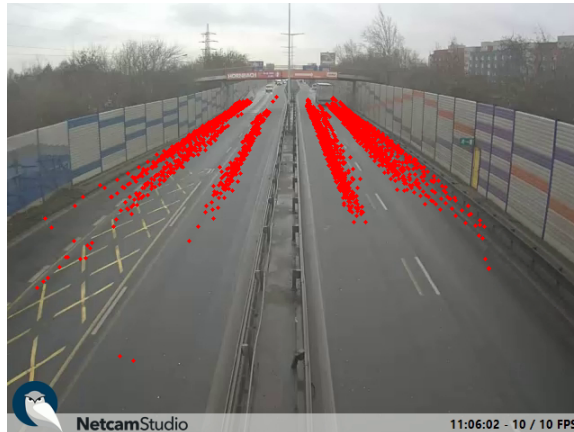
Figure 7.4: Radar and video pairs collected by the estimated intrinsic and extrinsic matrix method (AIEM)
