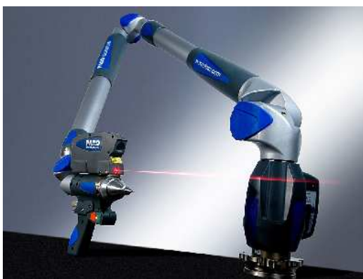
Obr. 3.5 Meracie rameno Faro 13 .
