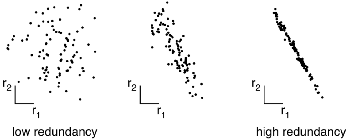
Fig. 1.32: Example of low and high redundancy between two variables r_1 and r_2 . The third is example of two highly correlated variables indicates high redundancy ( r_2 can be expressed as a linear combination of r_1 , i.e., r_2 = kr_1 ) [288].
