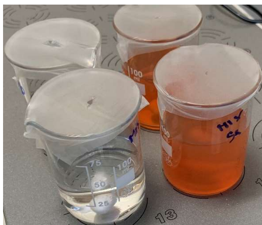
Figure 30: Samples prepared to undergo the polymerization, on the left side sample without selenium nanoparticles present, on the right side samples containing selenium nanoparticles.
