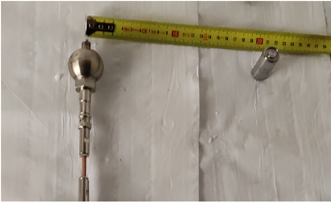
Fig. 6. Placement of the detector (left) and the neutron source (right) during the measurement
