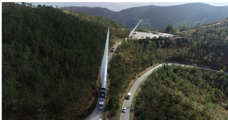
Obr. 7.8: Transport lopatky systému Blade Lifter [82].
