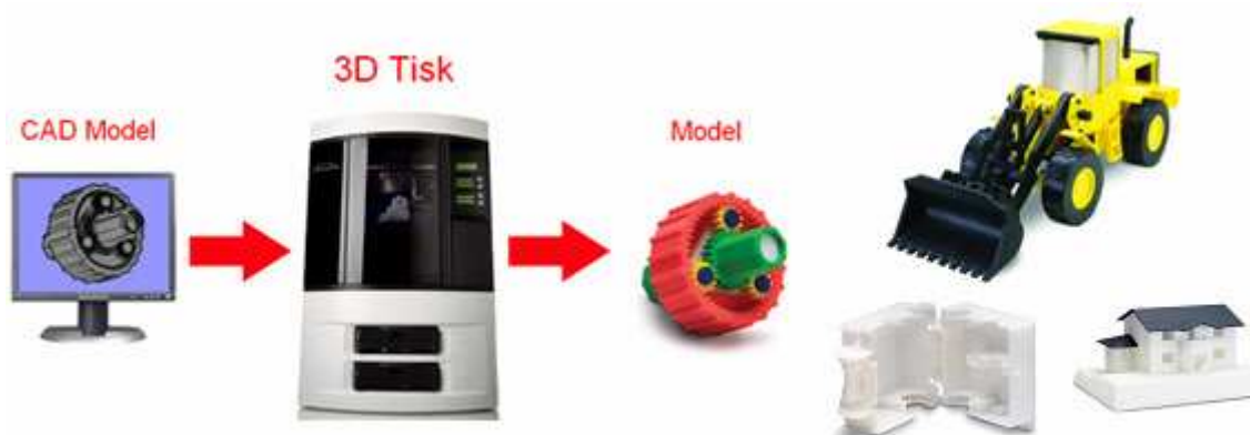
Obr. 6.1 Princip tvorby 3D modelu (24)
