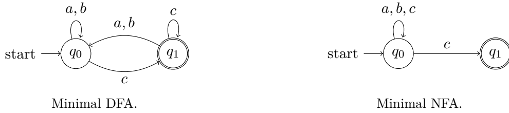
Figure 2.1: A comparison of the minimal forms of NFA and DFA for the regular language defined by the expression (a|b|c)^*c . In the DFA, each occurrence of the symbol c must be treated as a possible end of a word. However, if a or b follow c , it must transition back to the initial state. On the other hand, the NFA can nondeterministically guess that the symbol c is at the end of the word, allowing for a more compact representation.
