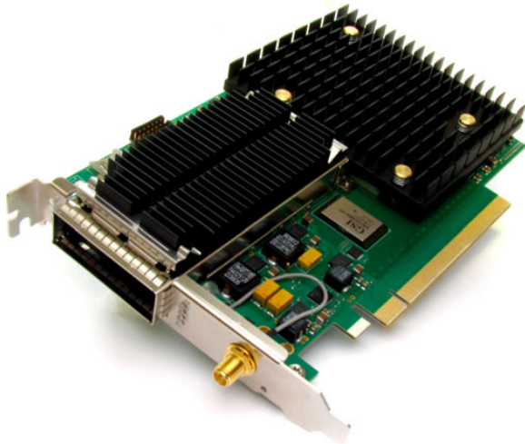
Fig. 10. COMBO-100 G accelerator used for our prototype implementation.
