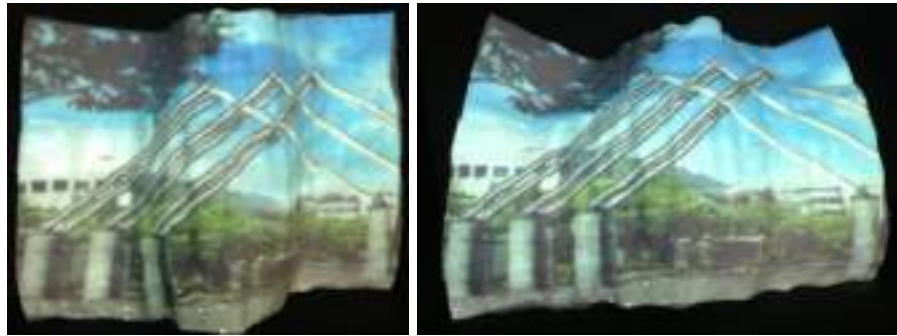
Figure 28: Results of texture projection. The same texture is deformed and projected onto differently deformed surfaces.
