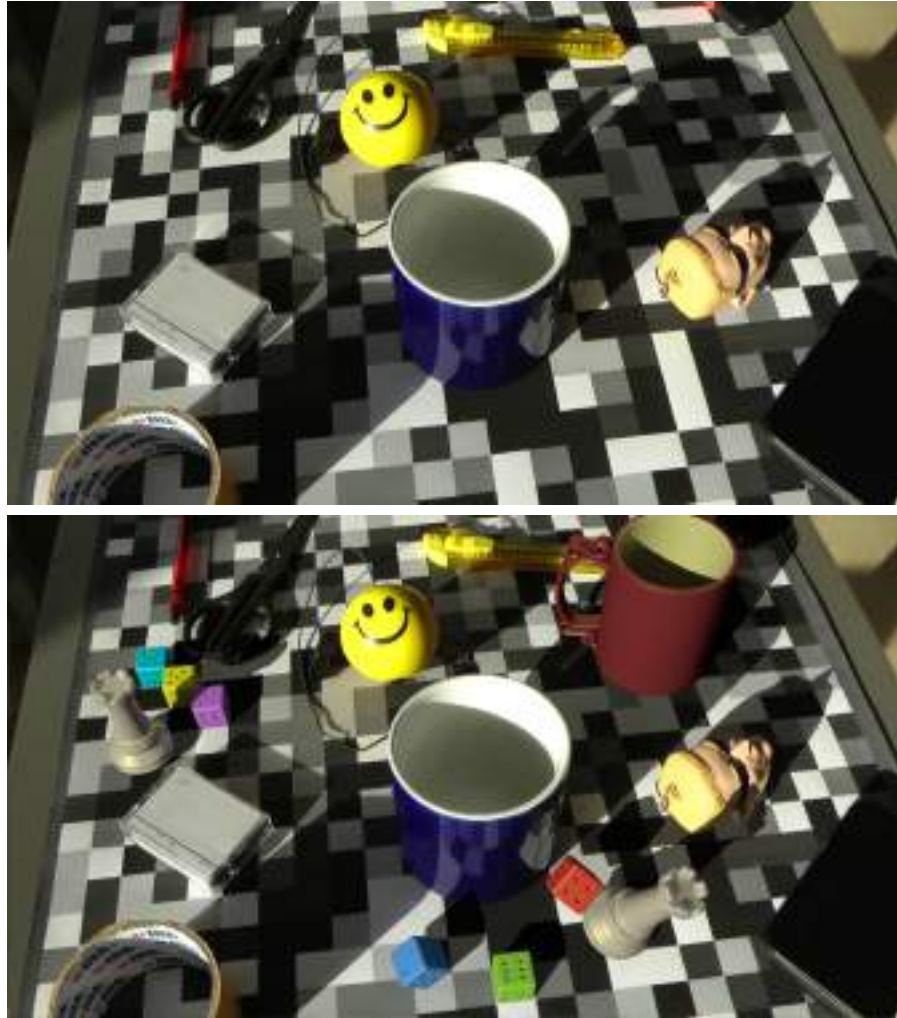
Figure 54: The use of Shades of Grey (SoG) marker field. Top: Original image – input to the detector. Bottom: Recognized camera location and augmented scene.
