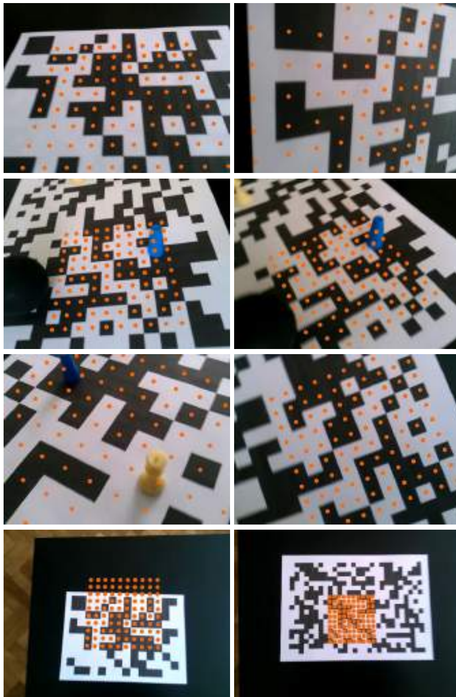
Figure 52: Sample images from the dataset taken with HTC Desire GSM ( 720 \times 480 ), HTC Evo 3D ( 720 \times 480 ) and HTC Titan ( 640 \times 480 ) smartphones. Orange dots are points x_{ij} sampled from the input image.
