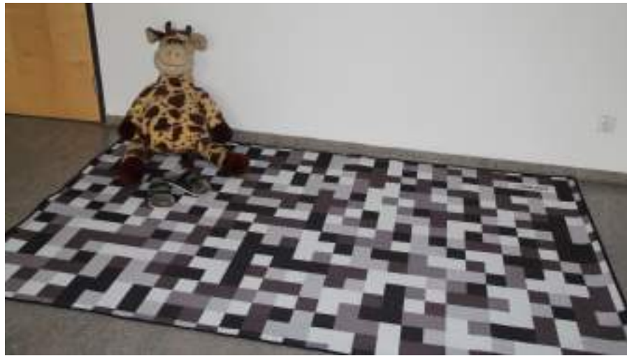
Figure 98: UMF carpet designed and manufactured for the Project reSound game (it has been of course used for another applications too). The carpet is 1.5 m wide and 2.4 m long with modules 7.5 cm big.
