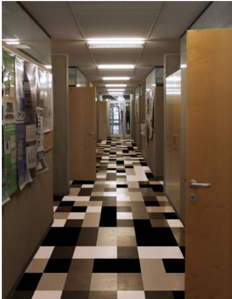
Figure 77: Greyscale UMF printed on the flooring can be used for indoor navigation by humans using augmented reality and/or by robots to precisely determine their position in the building.
