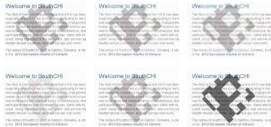
Figure 89: Examples of mixed-in marker field with varying presets. Top row: Different background blur radii. Bottom row: Varying opacity levels.
