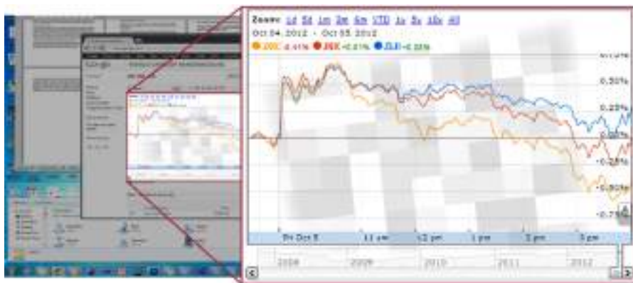
Figure 85: The goal of our work is to insert a subtle piece of information into the monitor screen that would be reliably detectable and could accurately establish the location within the screen observed by an ultramobile device (mobile phone, tablet. . .).
