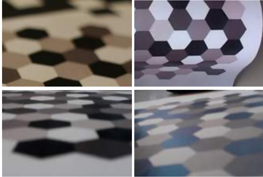
Figure 72: Examples of problematic edges (failure cases) within the pictures taken by a mobile phone of the marker field. The recognition can be challenging due to motion blur, uneven lighting conditions, high distortion, etc.
