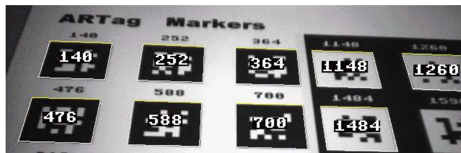
Figure 12: ARTag markers detected in an image. Overlaid with white border and ID shown above.
