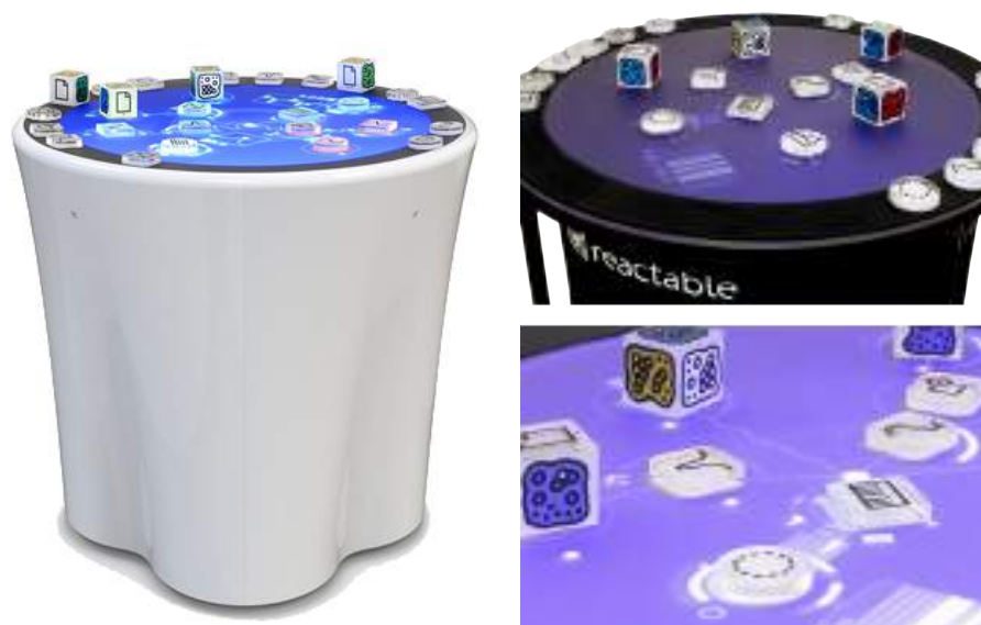
Figure 15: Left: Photo of entire reactTable. Right: Photos of reactTable with different “stones” embedded with markers on the bottom representing different sounds and instruments.
