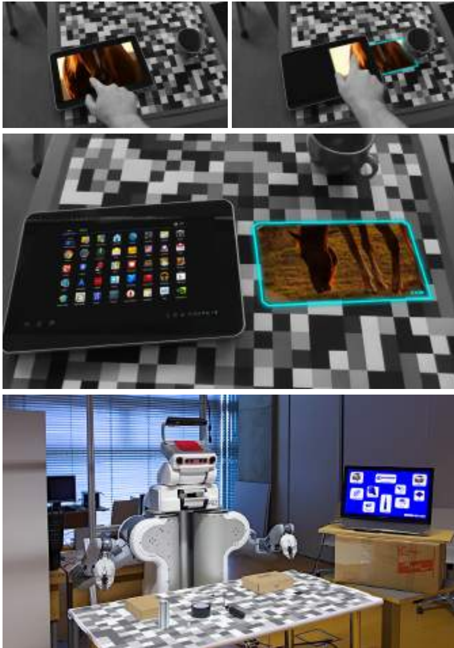
Figure 102: Tabletop interaction examples. The marker field covers the whole table surface and fosters the camera pose estimation.
