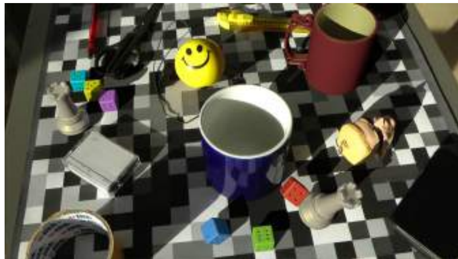
Figure 101: UMFs are highly resistant to occlusion and therefore are ideal for tabletop applications. Red cup, dices and chess pieces are augmented to the scene. Everything else is the original image.
