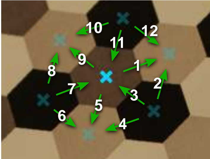
Figure 62: Identification of a fragment of the marker field based on the intensity differences between hexagons.
