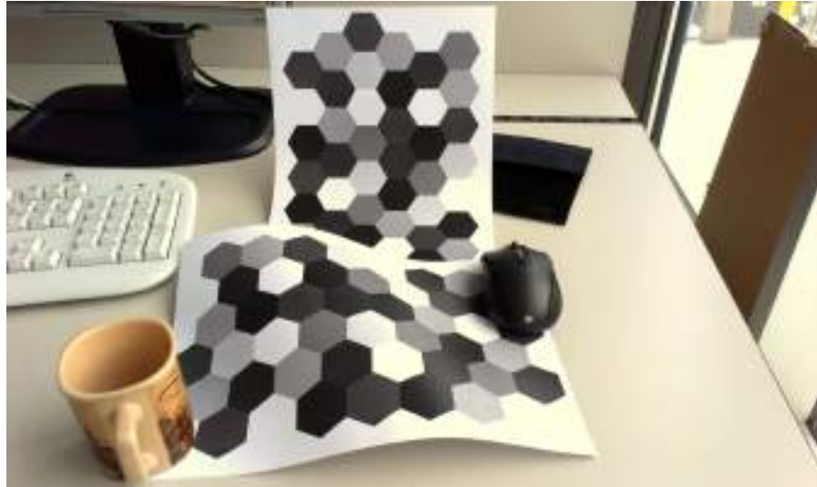
Figure 61: A camera snapshot of the deformed marker field in a realistic environment.
