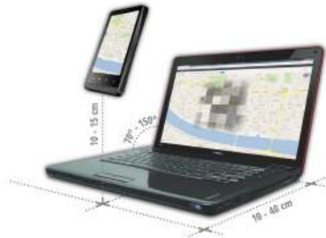
Figure 90: Parameters of marker detection reliability setup – distance between mobile device and laptop, range of screen angles used during tests and height range of a mobile device in order to be focused on the same point on screen.
