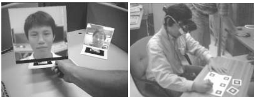
Figure 7: Demonstration of first intended use of ARToolKit (AR collaborating system). Left: Virtual monitors with the camera feeds from remote collaborators. Right: Person with HMD broadcasting his AR desktop.
