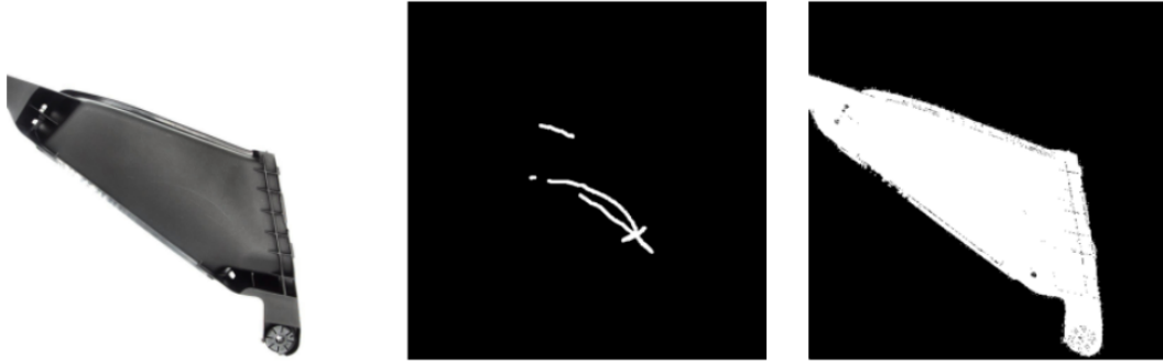
Fig. 28: Failure of the pixel-level classification despite great pixel-AUROC on Dataset-A image: Original image (left), Ground truth mask (middle), Predicted binary mask (right)
