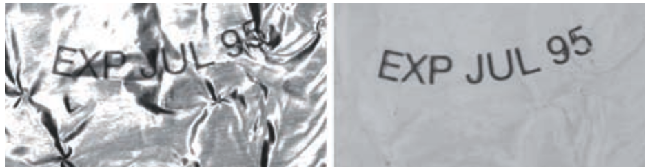
Fig. 2: Comparison of reflective surface illumination: ordinary bright field forward lighting (left) and a lighting with dome structure (right) [15]
