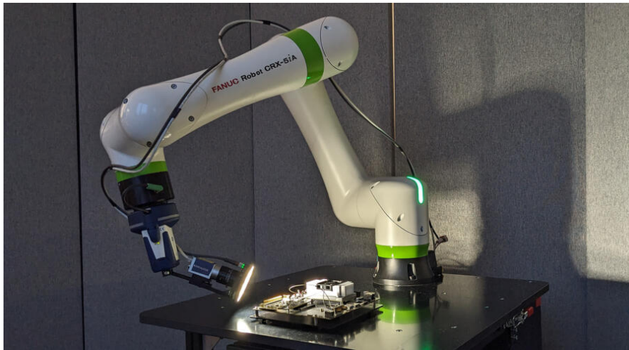
Fig. 6: Deep learning-based solution for final assembly quality inspection with collaborative robot [22]
