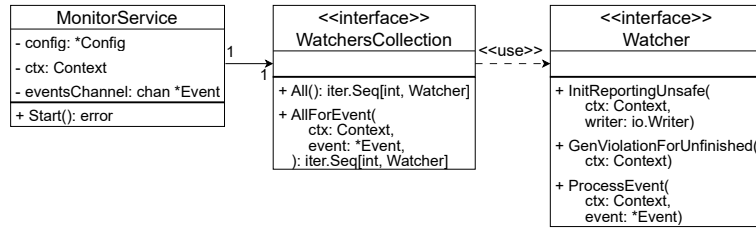
Figure 6.6: Class diagram representing the monitor service.
