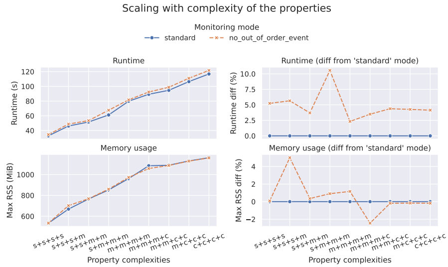
Figure 7.2: Visualization of the runtime and memory usage scaling in regards to the complexity of the properties.
