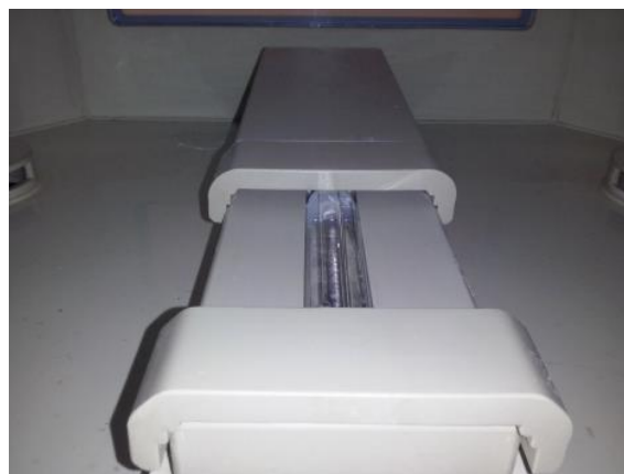
Pic. 4: Rotating string electrode in Nanospider NSLAB 500 Elmarco.
