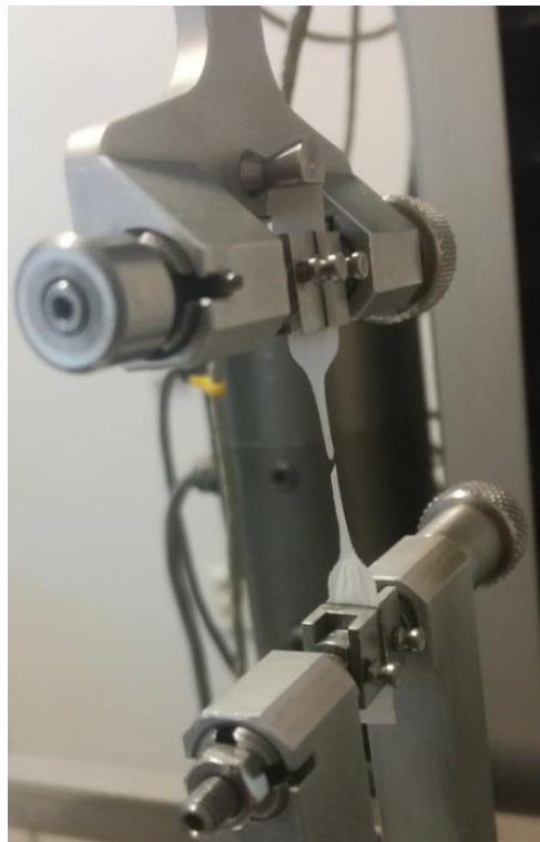
Fig. 9: Tensile testing of HA/Ag-NPs nanocomposite material with ZWICK Z 010, Zwick – Roell, 10 N measuring cell.
