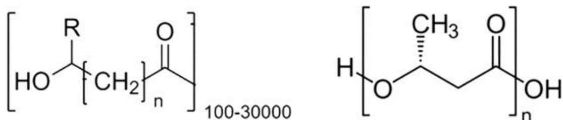
Figure 2 (a) The general molecular structure of polyhydroxyalkanoates; (b) P(3HB) molecule [13]
