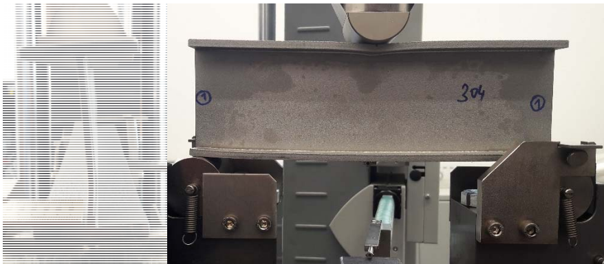
Fig. 1: Failed fatigue experiment of IPE80 profile – right buckling – left plastic deformation under the load.
