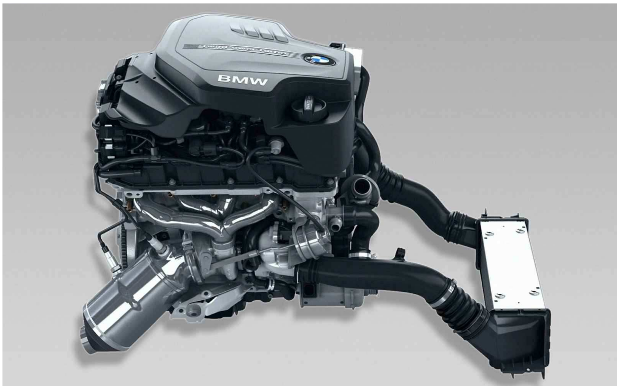
Figure 2 BMW's N20 four-cylinder engine with TwinScroll turbocharger [5]
