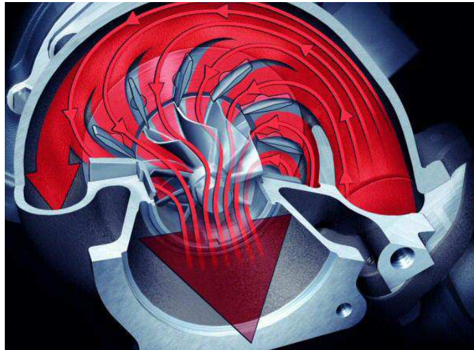
Figure 14 Open VNT mechanism [21]
