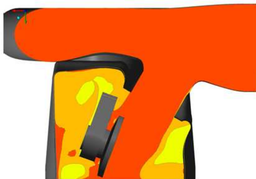
Figure 80 Flow vectors at 80deg open position
