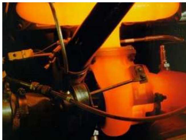
Figure 24 Gasoline turbocharger environment at full load [16]
