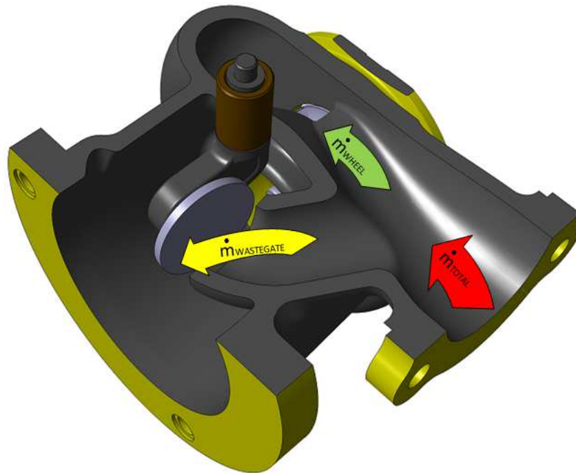
Figure 97 Section view (A-A) through wastegate channel
