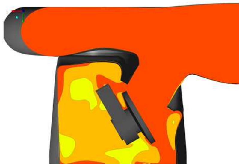
Figure 76 Flow vectors at 30deg open position
