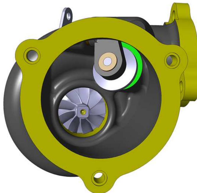
Figure 88 Discharge design with horizontal bushing axis
