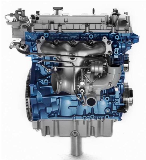
Figure 1 FORDS's GDTi 1.6 liter engine [4]
