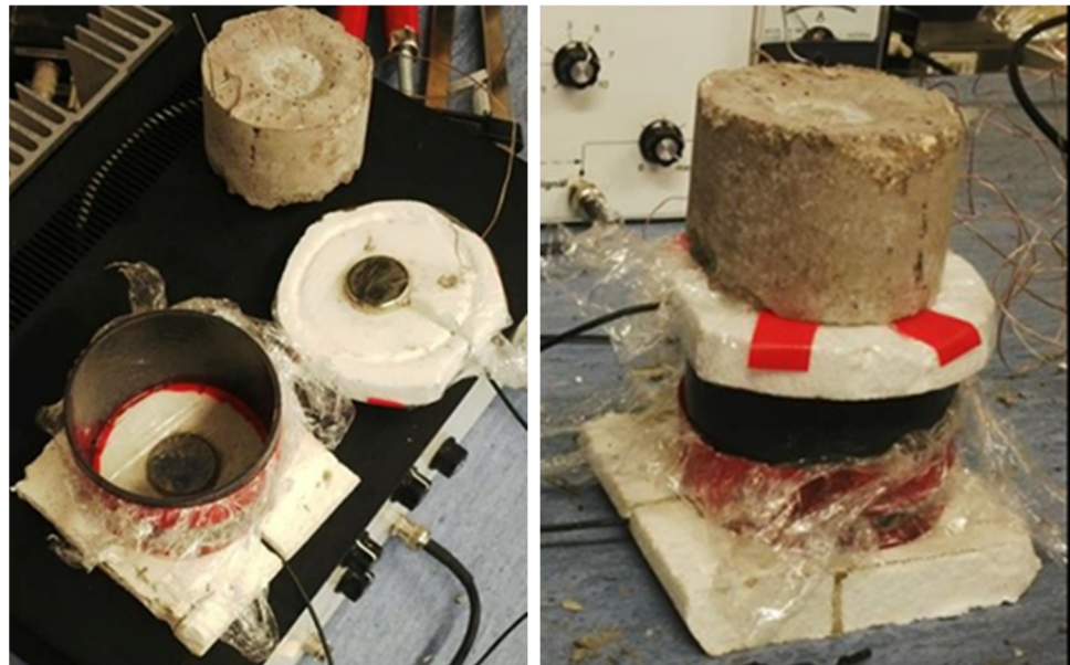
Figure 2. Plastic mould and polystyrene plates with piezoelectric sensors and during measurement (author).
