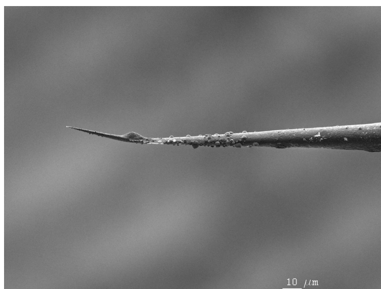
Fig. 8.3: The apex of a gold tip (carbon rod electrode, manual turn off, \text{CaCl}_2:\text{H}_2\text{O} , SE SEM picture).
