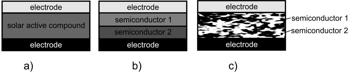
Fig. 5.4: Types of setups SC: a) single layer, b) bilayer, c) bulk active layer.
