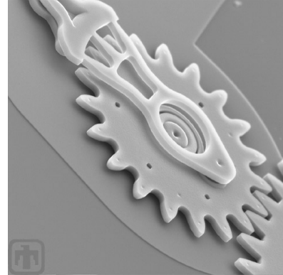
Figure 2.3: Close-up of micromotor with meshing gears. Source: [38].
