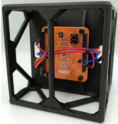
Figure 5.3: Second version of prototype dice from accelerometer shield side.
