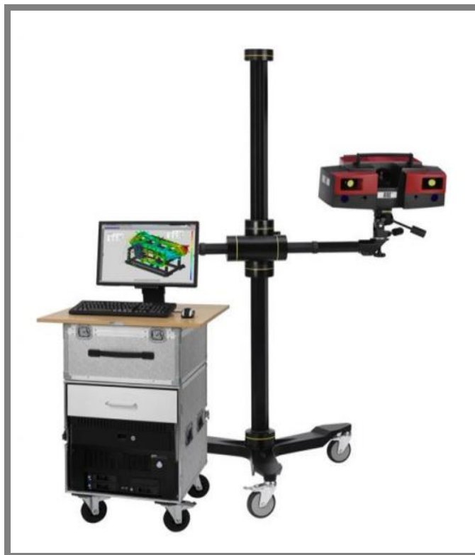
Obr. 13 Sestava ATOS Triple Scan III [1]
