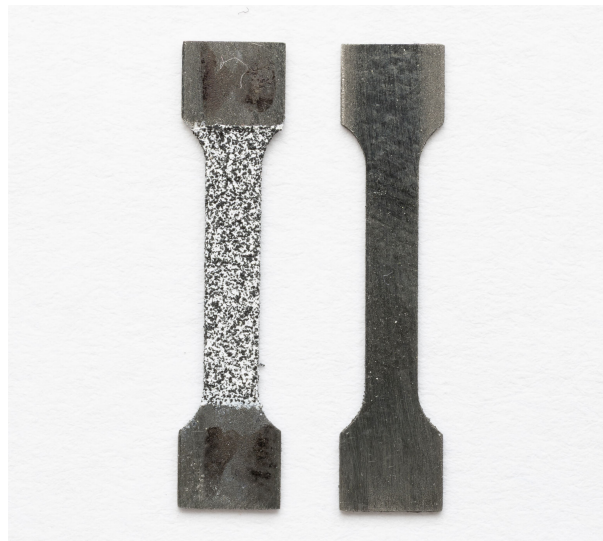
Figure 3.1: Unique pattern used on miniature specimen compared to the original surface [54]
