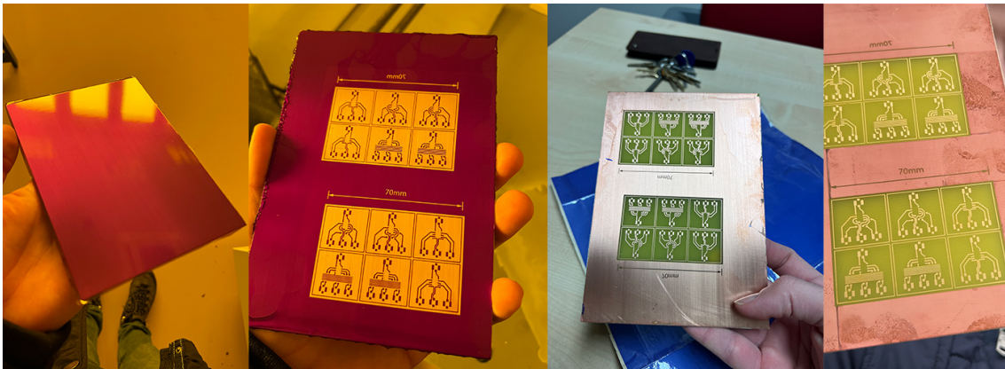
Fig. 3.11: Process of creating a custom PCB for sensor handling. First a photosensitive layer was laminated onto a one-layer PCB. An image of the design was exposed and developed.
