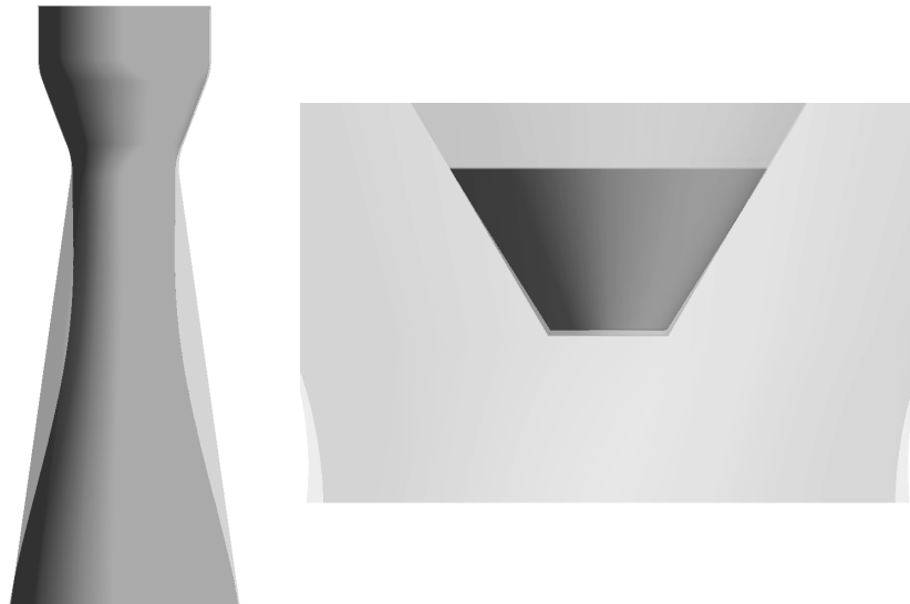
Figure 5.1: Results of the adjoint shape optimization, both the diffuser (left) and the hub (right) are shown, the initial shape is in light grey and final shape in dark grey
