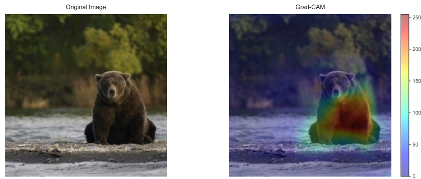
Figure 4.7: Grad-CAM: Class activation map generated using gradient-weighted importance of feature maps in a convolutional layer (right). The original image (left) is from the ImageNet dataset [14], and the saliency map was computed using the VGG16 network [59].
