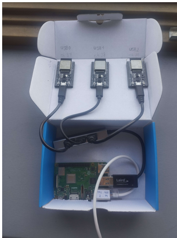
Figure 5.2: Physical implementation of the ESP32-based monitoring probe
