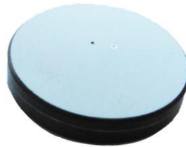
Fig. 14: DLC coated sample
