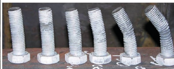
Fig. 13 Deformed shape of the connection at 450 °C: a) test and b) CBFEM
