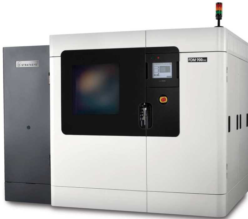
Obr. 7 FORTUS 900mc, technologie FDM [19]
