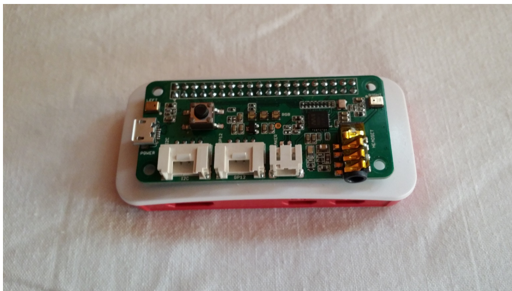
Obr. 4.1: ReSpeaker 2 Mics Pi HAT na Raspberry Pi Zero
