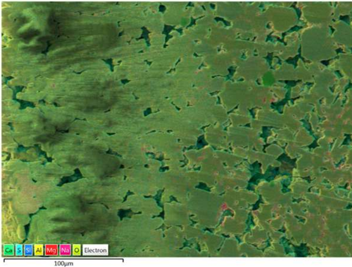
Figure 20: Layered image from the individual EDS analysis of GGBFS-based specimen.
