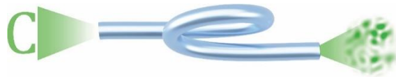
Figure 2.1: Coherent light coupled to the MMF exits as a speckle pattern due to different phase velocities of different propagating modes.
