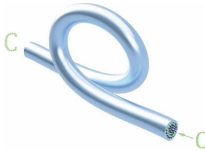
Figure 1.3: Transmission of the image in the fibre bundle consisting of many spatially separated cores. The light from the letter C is propagating only through the spatially separated cores placed within the cladding, all packed within one probe.
