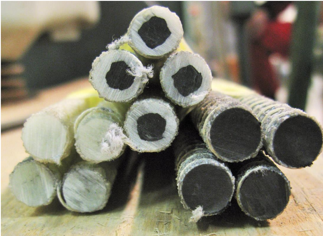
Obr. 6 - GFRP (Glass Fiber Reinforced Polymer), C-GFRP (Carbon-Glass Fiber Reinforced Polymer) a CFRP (Carbon Fiber Reinforced Polymer) výztuž do betonu [25]
