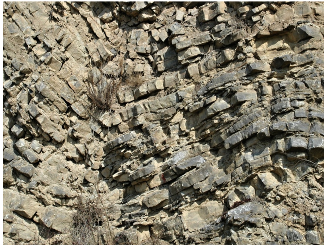
Fig. 1. The network of rock joints that was uncovered during excavation work at lime quarry Hády near to the city of Brno Czech Republic.
