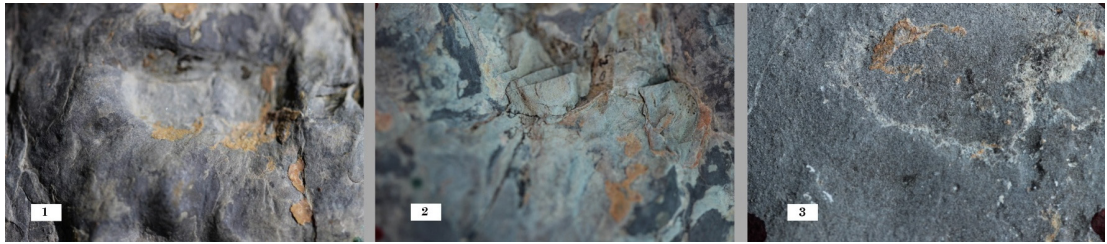
Fig. 4 Database surfaces of limestone samples 1, 2 and 3 that serve for similarity comparisons with investigated surfaces. The database JRC values are assigned to the investigated surfaces on the similarity basis.
