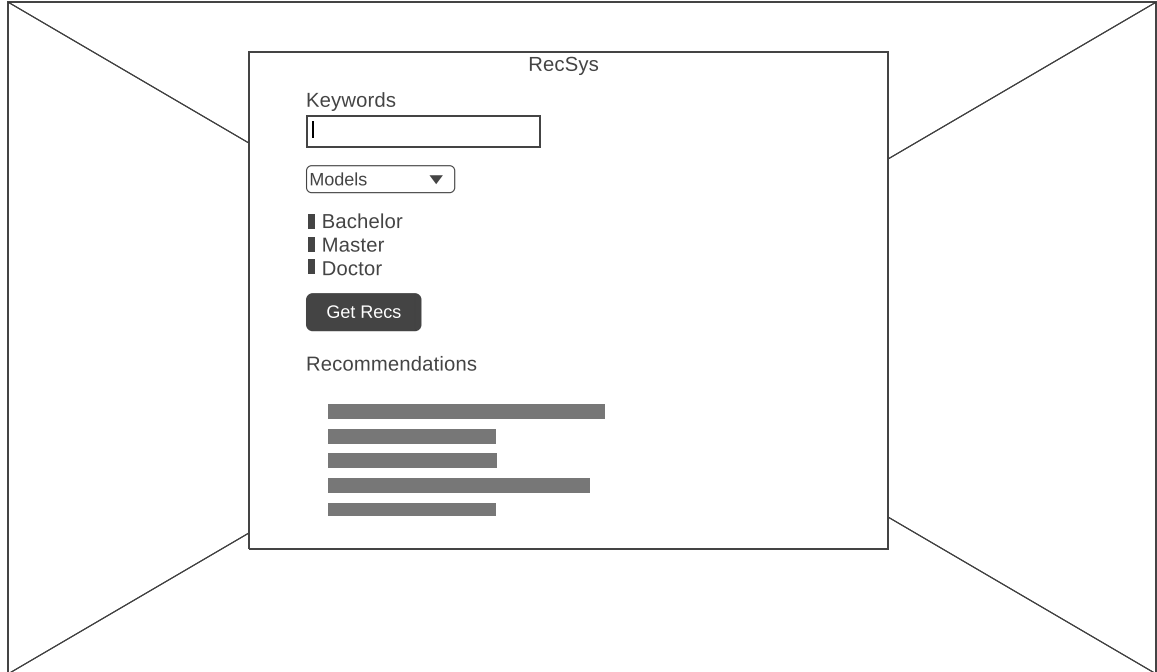
Figure 4.1: Wireframe of the user interface, illustrating the input field for text, model selection options, filtering by type of work, and a button to generate results. The output is displayed in a dedicated Recommendations section.
