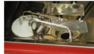
Continuously wetted, self cleaning psychrometric humidity sensor, temperature measuring sensor, test specimen protection
