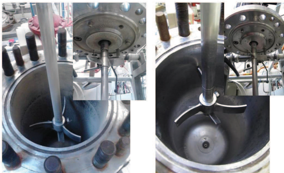
Figure 23: Catalyst depositing in the 6 L vessel (left section) and its elimination by Atmer 163 surface active agent (right section).
