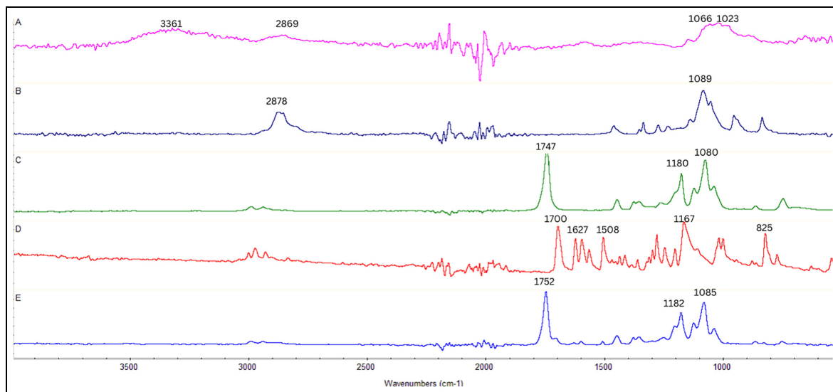
Figure 2. FT-IR spectra of CS (A), PEG (B) PLA (C), EPMC (D), and the nanofibers (E).
