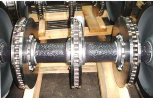
Figure 9 Example of coated axle [44]
