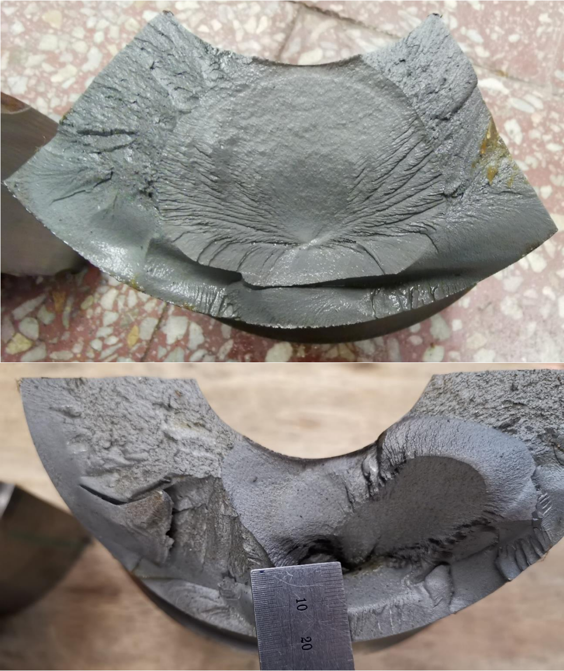
Figure 91 Different railway axles fractured by the internal fatigue crack growth.
