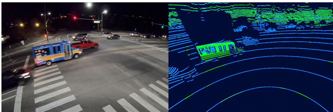
Figure 2.3: Example of LiDAR camera used for smart traffic management Source: [23]
