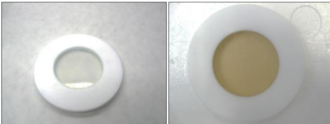
Figure S1. Plastic ring holder filled with in-situ gelatinized AG (left) and AG – HA (right) hydrogels, respectively.
