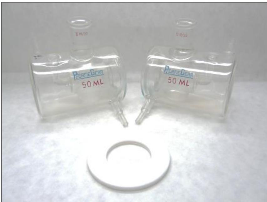
Figure S4. Side-by-side diffusion cells (PermeGear, Inc.)
