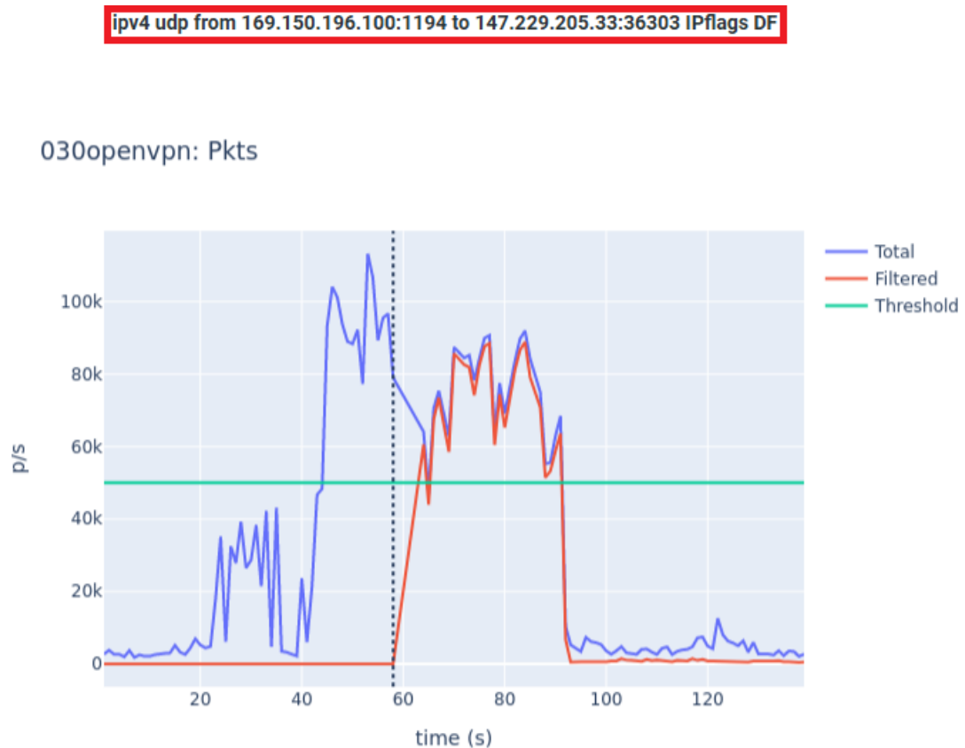
Figure 4.3: Final attack evaluation by DDoS-Guard, used to compare results with the developed tool
