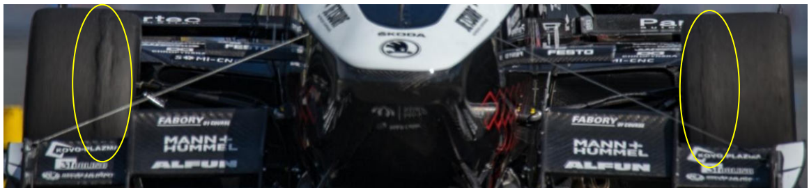
Figure 15 Visible piling up of rubber on the inner part of the C19 tires
