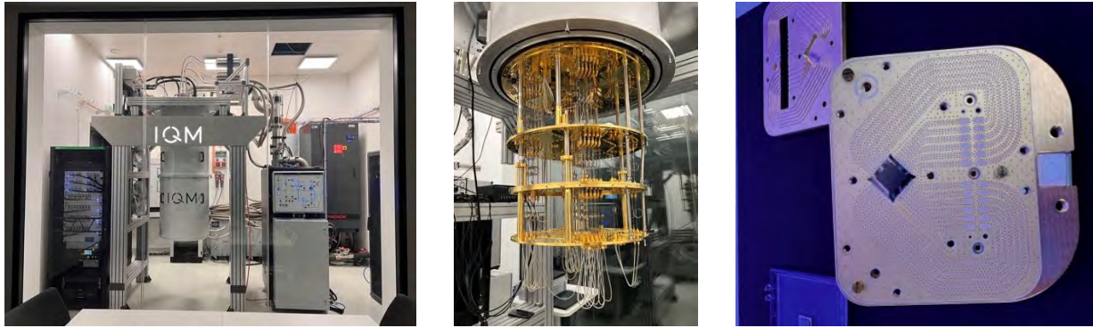
Fig. 5: VLQ quantum computer, its cryostat and quantum chip.
