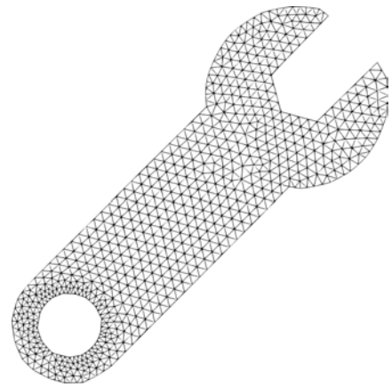
Fig. 4 Triangulation of a wrench
